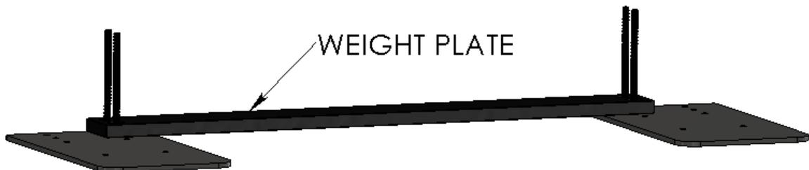
FOUR THREADED RODS INSERTED IN REAR INNER POST PLATE HOLES
